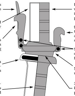
Ball and socket shanks decrease wear, kinking and binding of hoses, increasing hose longevity and pump performance.
