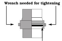
Flat Gasket can cause leakage
